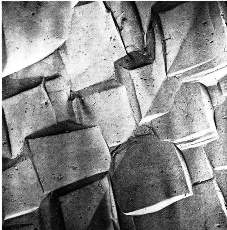
Fig. 2. Electron micrograph of germanium bicrystal. Angle of tilt \Theta=20^\circ . Specimen etched with RCA No. 2 etch solution to reveal (100) planes. (Magnification 5,430 ×; scale: |\text{—}| = 1\text{ }\mu .) Direct carbon replica pre-shadowed with platinum metal at approximately 27^\circ .
